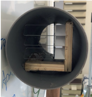
Fig. SA4.4 Picture of the microscope slide holder inside the cylinder of the spore trap. The holder can hold three microscope slides at a 45 degree angle.
